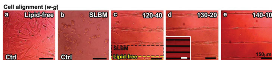
Figure 4. Incubation of HLF cells on SLBM patterned template. (a) HLF cell adhesion in random directions on S-PDMS transferred hydrophobic surface. No SLBM (lipid-free) is prepared prior to the cell incubation. (b) No adhesion of HLF cell was monitored on SLBM fully covered substrate. (c–e) Cell adhesions occur solely on hydrophobic (= S-PDMS) regions with controlled HLF cell alignment in w - g ; 120 \mu\text{m} – 40 \mu\text{m} (c), w - g ; 130 \mu\text{m} – 20 \mu\text{m} (d; inset for SLBM pattern), and w - g ; 140 \mu\text{m} – 10 \mu\text{m} (e). All scale bars: 150 \mu\text{m} .
